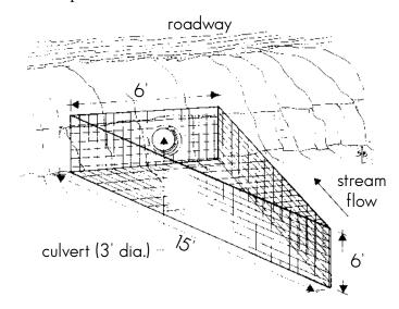
Triangular screen mesh design Constructed from 2" mesh welded wire: placed on upstream end of culvert: should be removed during winter to prevent ice damage. Dimensions shown are for a 1 meter culvert, increase measurements if required. (Drawing not to scale).
