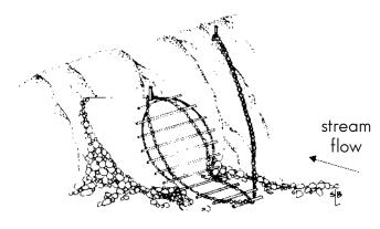
**Culvert protector-cleaner** Constructed by welding steel rods (4 inches apart) across a looped chain: upper end is held by a bolt placed through the top of the culvert; tail end is looped back and anchored on road bank; end of chain can then be attached to a vehicle and the grill flipped up onto the road to clear culvert
