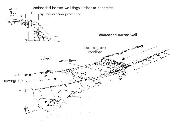
Low water crossing If we can accept the fact that a road will experience periodic flooding, then the road can be designed to receive the flowing water with minimal or no damage.
