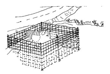
If beavers do begin to construct a dam against a fence installed to protect a culvert, it may then be necessary to install a WLCD to regulate the water level. The deep-water fence protecting the culvert will act as an emergency spillway during high run-off conditions when the WLCD cannot handle the flow. (Note: Road grades cannot usually be used as dikes. Deposited debris may have to be removed or modified.)
