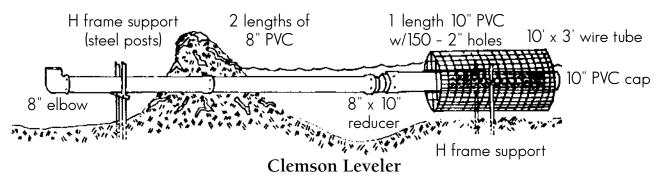
2. Two features are required to help reduce the sensation of water flowing. First, the intake has 150 2inch holes drilled into the 10-inch PVC which is protected by a 3-foot diameter wire pipe exclosure. Second, the 10-inch diameter intake device is reduced
